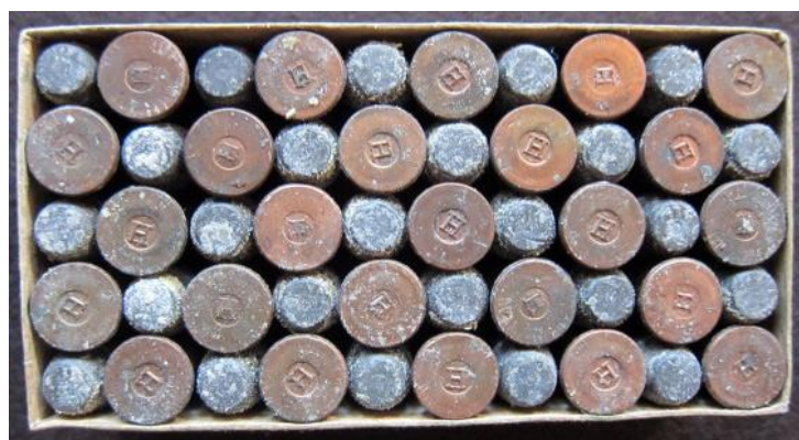
Figure 1. The copper base of this .44 caliber Henry Flat rimfire cartridge has a raised and serified “H” headstamp in a recessed circle. The red arrow points to the lead bullet’s single grease groove or cannelure. Source: https://en.wikipedia.org/wiki/.44_Henry . Figures 2, 3. Original cardboard box containing fifty .44 caliber Henry Flat rimfire cartridges manufactured by the Winchester Repeating Arms Company. Source: Clarks Antiques, https://clarksantiques.com/ammo/44-henry-flat-rimfire/ .
