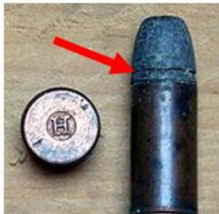
Figure 1. The copper base of this .44 caliber Henry Flat rimfire cartridge has a raised and serified “H” headstamp in a recessed circle. The red arrow points to the lead bullet’s single grease groove or cannelure. Source: https://en.wikipedia.org/wiki/.44_Henry . Figures 2, 3. Original cardboard box containing fifty .44 caliber Henry Flat rimfire cartridges manufactured by the Winchester Repeating Arms Company. Source: Clarks Antiques, https://clarksantiques.com/ammo/44-henry-flat-rimfire/ .
